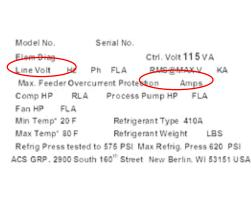
• Check the transformer primary voltage connections to be sure they are configured for the electrical power you are using. The voltage at the main power connection must read within plus or minus ten percent (±10%) of the voltage listed on the serial tag. Electrical connections must conform to all applicable codes.
